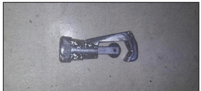
Fig. 3: Tube Cutter Used in Present Experiment
