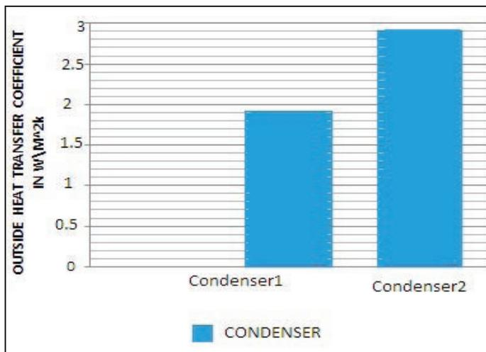
Fig. 7: Outside Heat Transfer Coefficient for Existing Condenser and Spiral Coil Condenser
