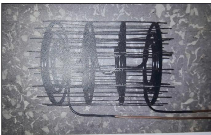
Fig. 6: Spiral Coil Condenser Used in Present Experiment
