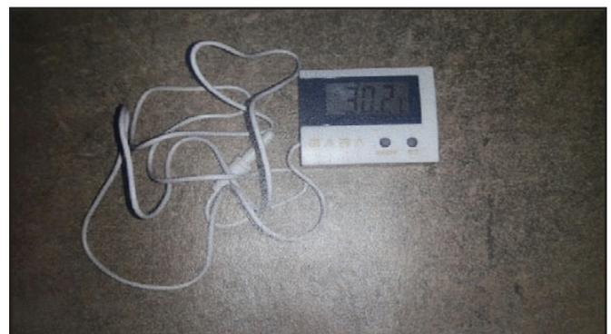
Fig. 4: Digital Thermometer Used in Present Experiment
