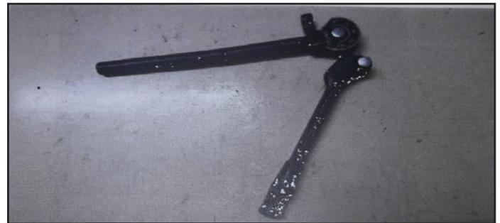
Fig. 2: Tube Bender Used in Present Experiment
