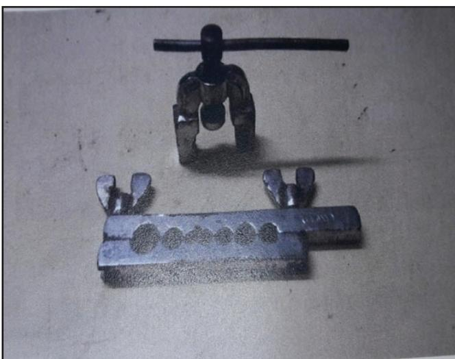
Fig. 1: Flaring Tool Used in Present Experiment
