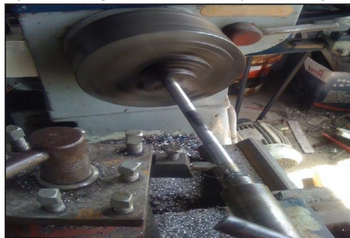
Fig. 5: Shows Preparations of Specimens on Lathe Machine
