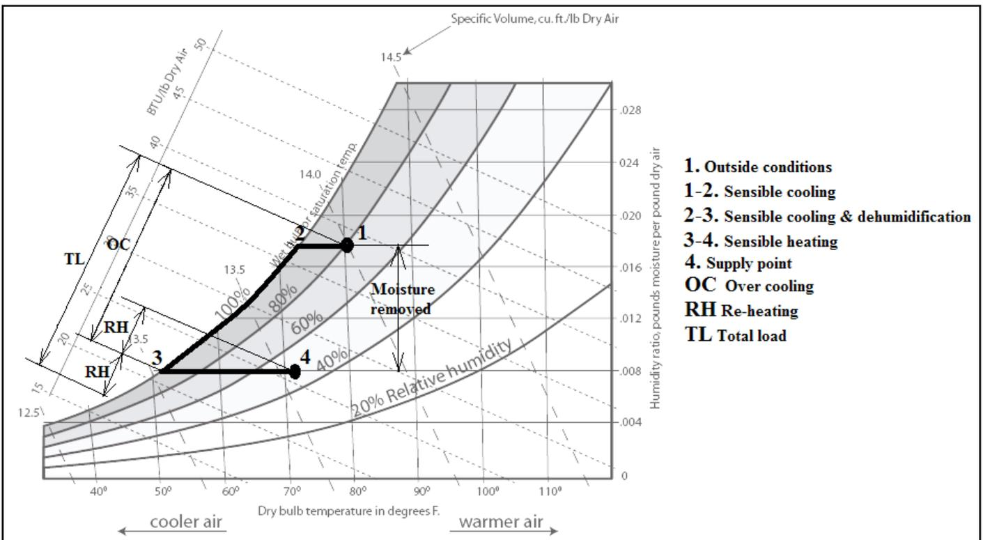
Fig. 1: Conventional Dehumidification & Cooling of Air Shown in Psychrometric Chart
