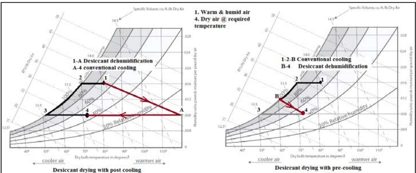
Fig. 5: Hybrid Dehumidification & Cooling System Combination of Conventional & Desiccant Dehumidification System
