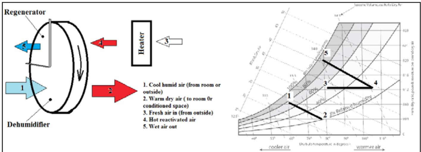
Fig. 3: Solid Desiccant Dehumidification
