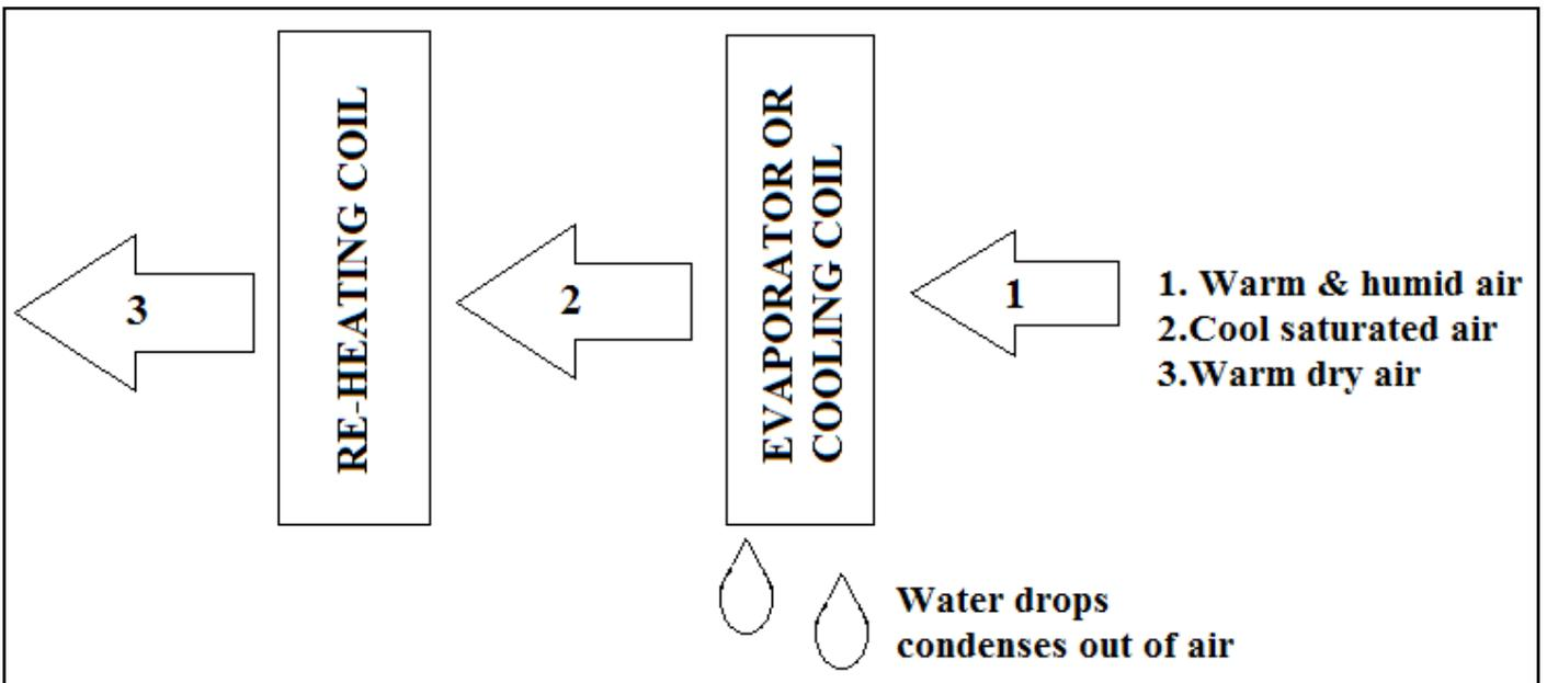
Fig. 2: Conventional Dehumidification & Air Conditioning
