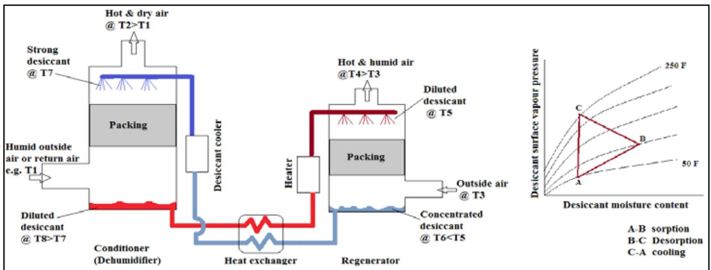
Fig. 4: Liquid Desiccant Dehumidification
