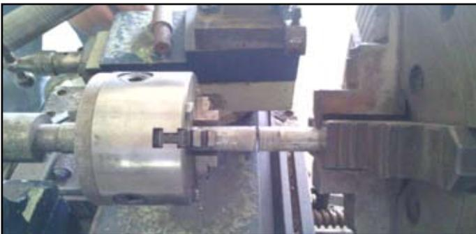
Fig. 1: Fitting of Work Pieces on Chuck and Threw Chuck
