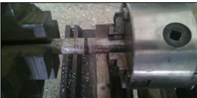
Fig. 2: Friction Welding Joint
