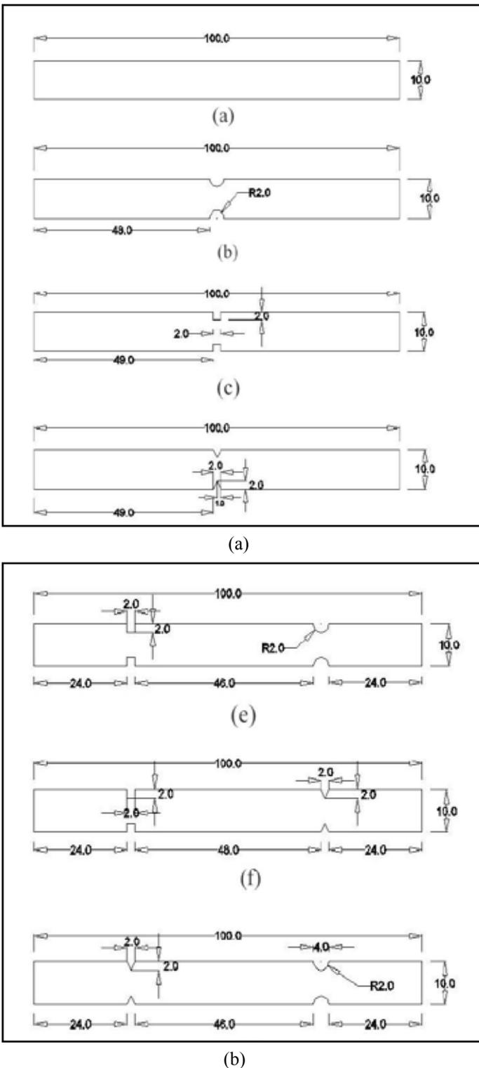
Fig. 1: Geometry of Different Types of Baffle Arrangements
