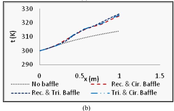
Fig. 5: Temperature Variations Along the Center Line in Case of Double Baffle Used W.R.T no Baffle (a) Al, (b) Cu
