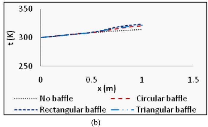
Fig. 4: Temperature Variations Along the Center Line in Case of Single Baffle Used W.R.T No Baffle (a) Al, (b) Cu
