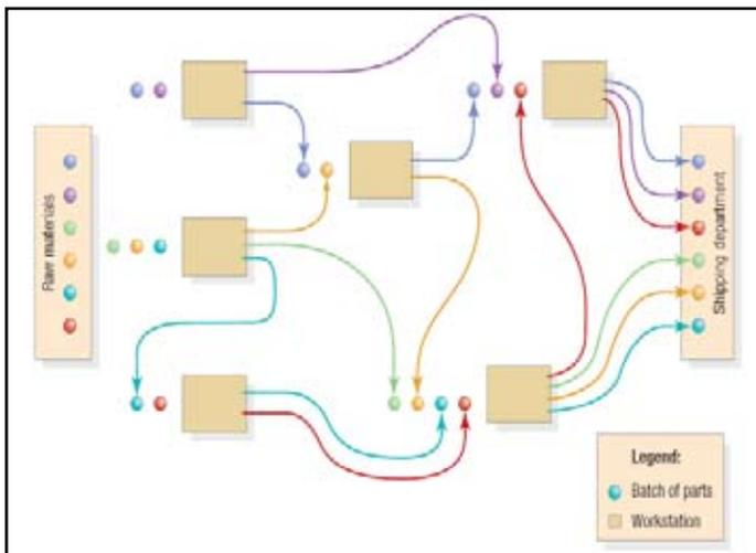
Fig. 1: Diagram of a Manufacturing Job Shop Process
