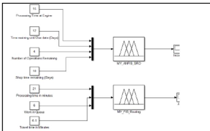
Fig. 10: Actual Simulation Model Developed for the Work
