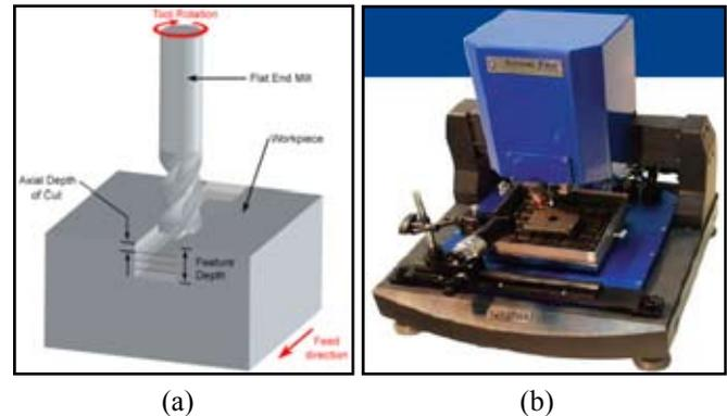
Fig. 1: (a). Basic End Milling Operation, (b). Three Axis-Vertical-Micromilling Machine -53725-2505939 [6]
