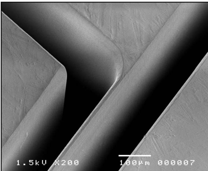
Fig. 7: Machined Micro Components With AlCrN Coated Cutting Tool [5]
