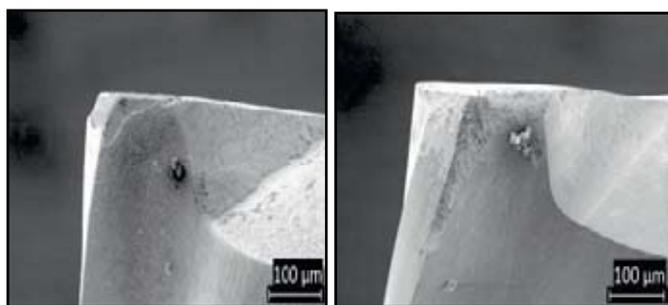
Fig. 4: (c). TiN Coated Tool, (d) TiAlN Coated Material After 2mm Depth of Cut [4]
