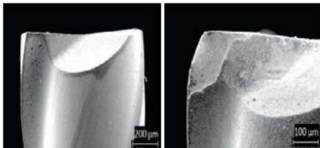
Fig. 4: (a). New Cutting Tool, (b) AlCrN Coated Tool After Machining of 2mm Depth of Cut [4]
