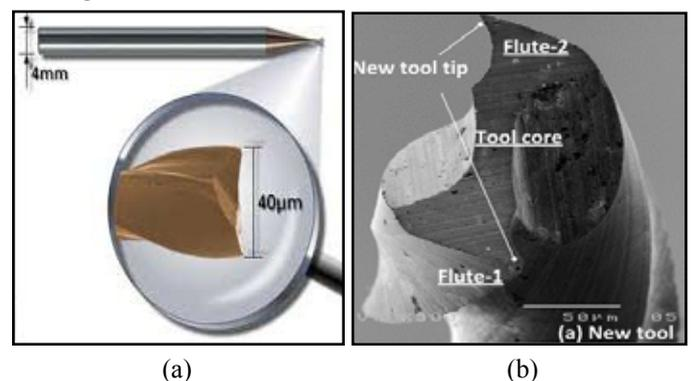
Fig. 2: (a). End Milling Cutter With 4mm Dia. [1] (b) SEM Image of End Cutter [2]
