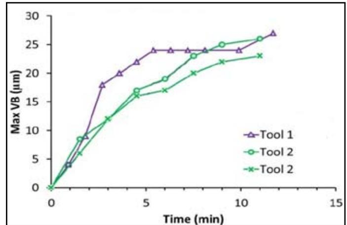
Fig. 5: Maximum Tool Wear Graph by Using Three Different Coated Tools [6]
