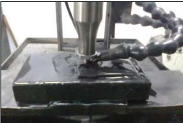
Fig. 1: Ultrasonic Drilling Machine AP-500 (Sonic Mill, USA)
