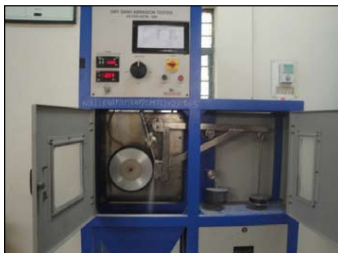
Plate 2 Three body abrasion test set up
