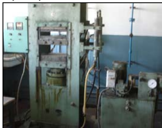
Plate 1 Compression moulding Hot press
