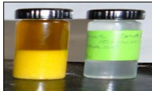
Fig. 8 & 9: Left Shows the Biodiesel and Water Samples Taken 2 Minutes Into the Continuous Washing, Right Shows the Effluent Samples Taken at the 10 Minute Mark
