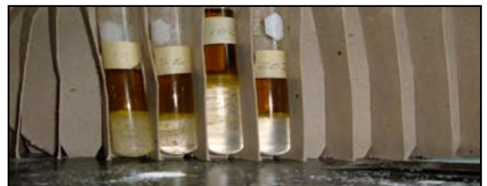
Fig. 10: Emulsions Left Over With Different Levels of Salt Concentration (Increasing From Left to Right).
