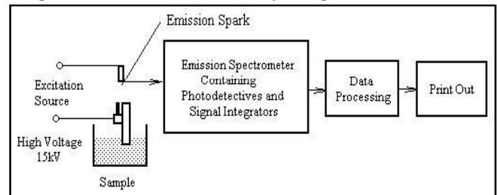
Fig. 1: Schematic Illustration of the Emission Spectrometric Analysis
