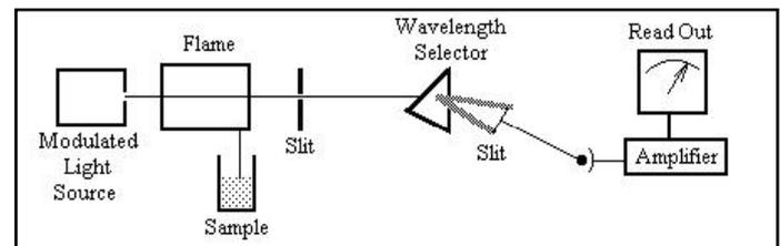
Fig. 2: Schematic Illustration of the Atomic Absorption Spectrometric Analysis
