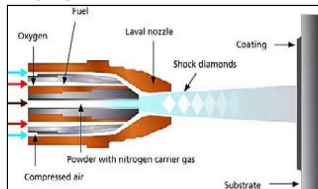
Fig. 1: High Velocity Oxy-Fuel [1]
