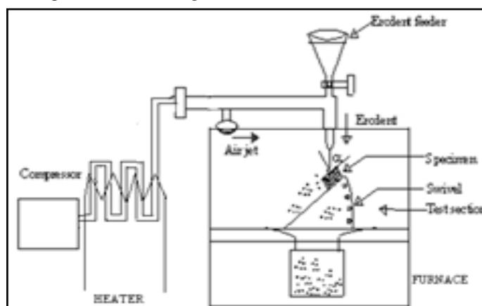
Fig. 3: Working Principle of Erosion Testing Machine
