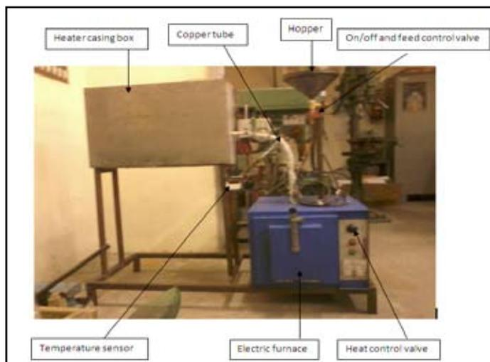
Fig. 2: High Temperature Air Jet Erosion Testing Machine
