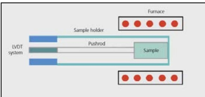
Fig. 1: Schematics of NETZSCH DIL 402 PC Dilatometer
