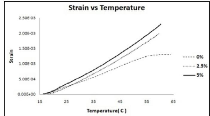
Fig. 2: Strain Variation With Temperature for Pure PMMA (0wt%), 2.5wt% MWCNT/PMMA and 5wt% PMMA/MWCNT Composite
