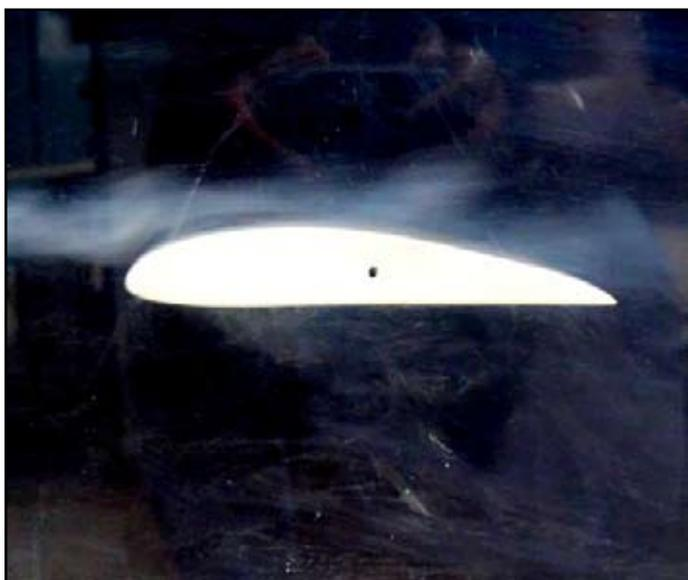
Fig. 6(b): Real Time NACA 4413 airfoil at AOA = 0°
