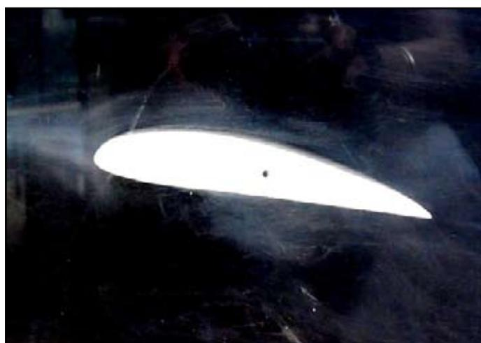
Fig. 8(b): Real Time NACA 4413 airfoil at AOA = 5°
