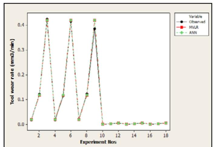
Fig. 2: Comparison Between Observed and Predicted Results of TWR Using MVLr and ANN
