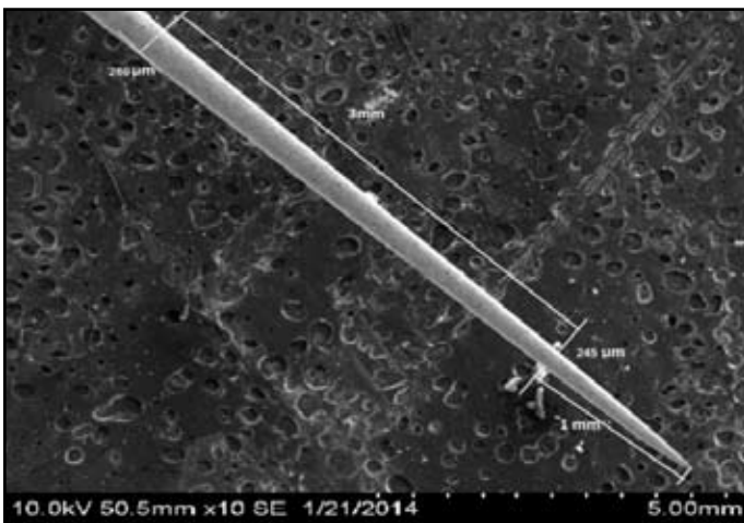
Fig. 4: SEM View of Micro Tool After Lapping Process
