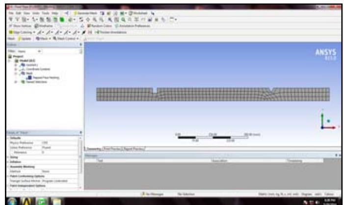
Fig. 5: Meshing for Rectangular Baffle
