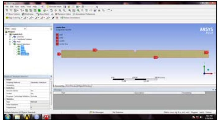
Fig. 4: Boundary Conditions for Triangular baffles
