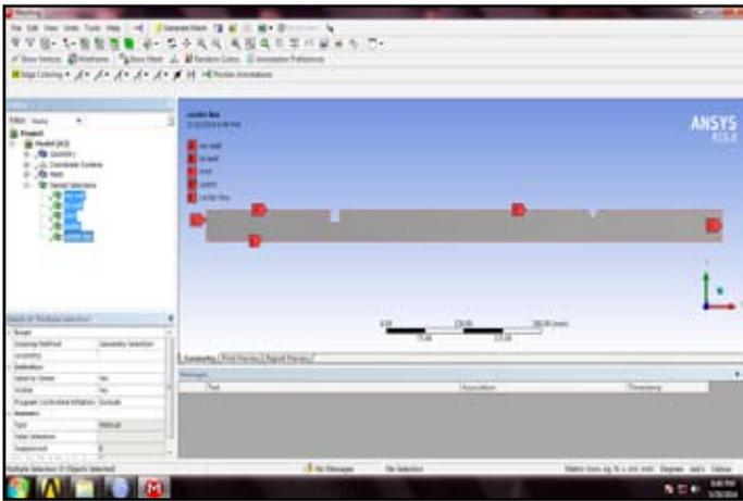
Fig. 2: Boundary Conditions for Rectangular Baffle
