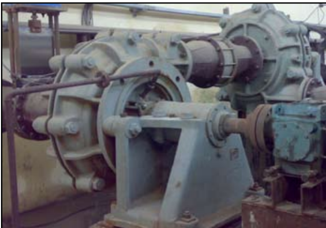
Fig. 1: Centrifugal Slurry Pumps in Series
