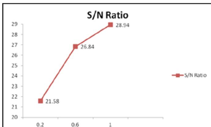
Fig. 3: Graph of S/N ratio for depth of cut (Smaller is better)
