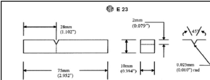
Fig. 3: Specimen for Izod Test
