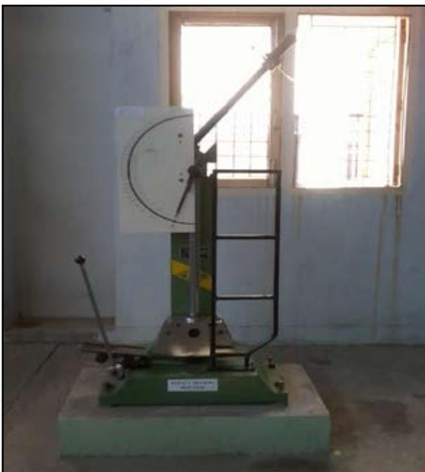
Fig. 5: Impact Strength Testing Machine
