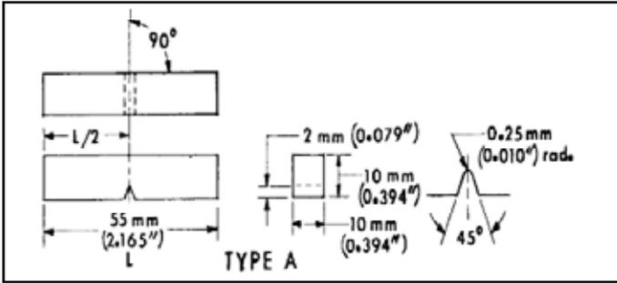
Fig. 2: Specimen for Charpy Test
