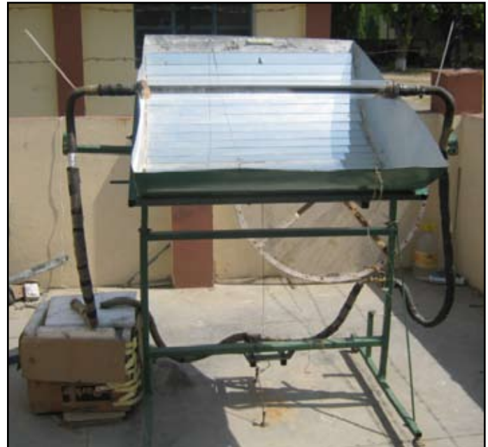
Fig. 1: Parabolic Trough Solar Collector (PTSC) set-up
