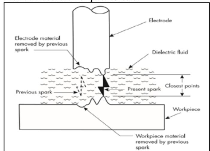
Fig. 2: How EDM Works
