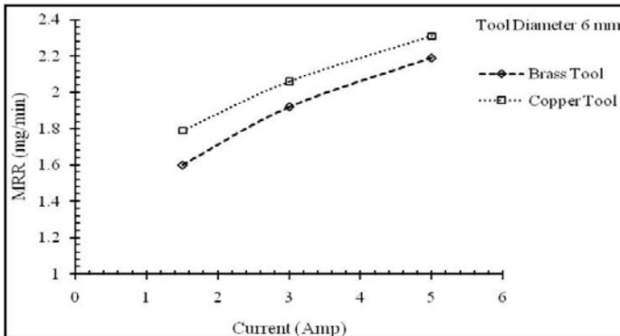
Fig. 7: MRR Versus Current for 6 mm Tool Diameter
