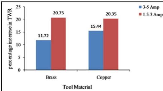
Fig. 13: Percentage Increase in TWR for Brass and Copper Tool Materials
