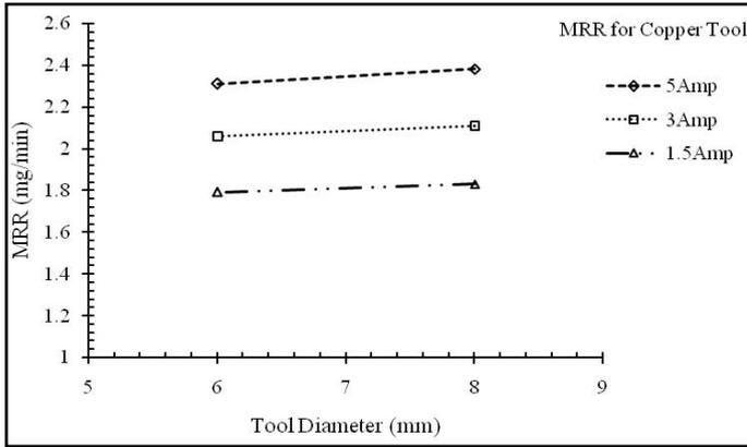
Fig. 6: MRR for Copper Tool
