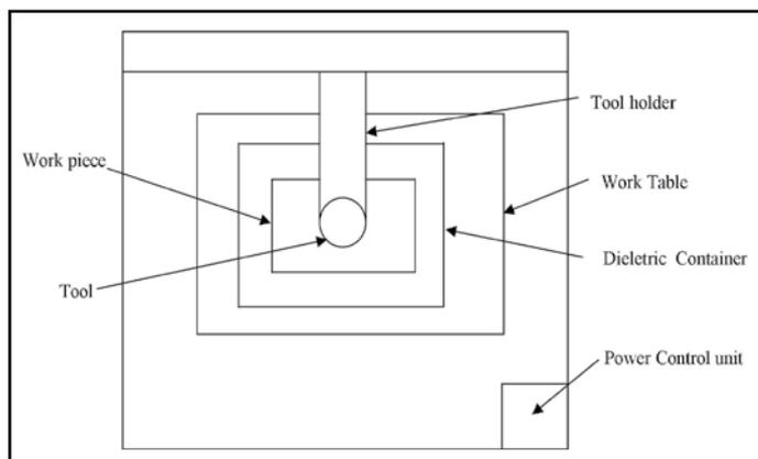
Fig. 3: Block Diagram of EDM
