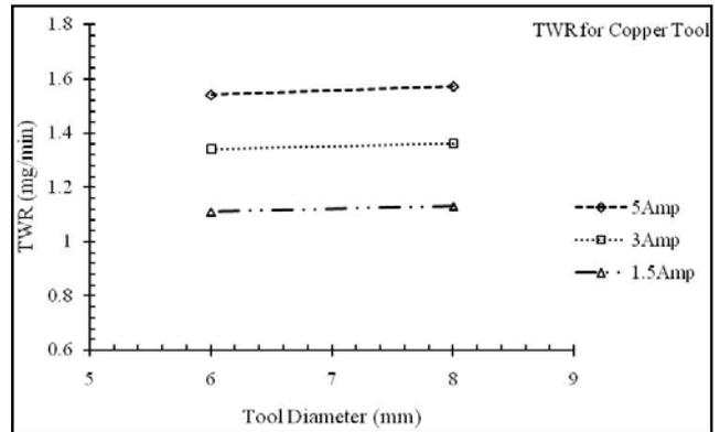
Fig. 10: TWR for Copper Tool
