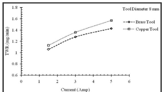
Fig. 12: TWR versus Current for 8 mm Tool Diameter
