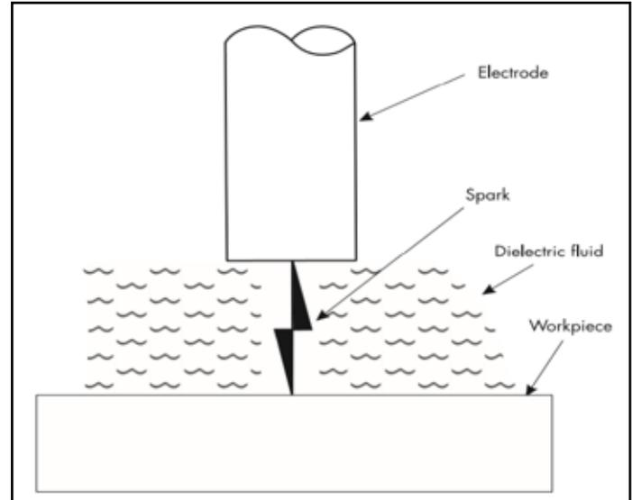
Fig. 1: Basic Components of EDM
