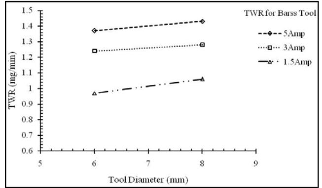
Fig. 9: TWR for Brass Tool
