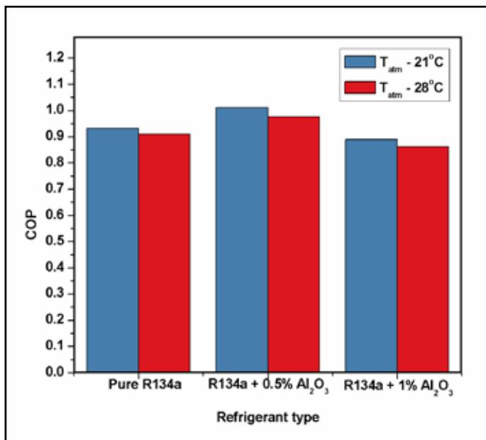
Fig. 3: COP Comparison for 6.5 LPH Volume Flow Rate, Evaporator Load at 30-31°C Operating at Ambient Temperature 21°C and 28°C
