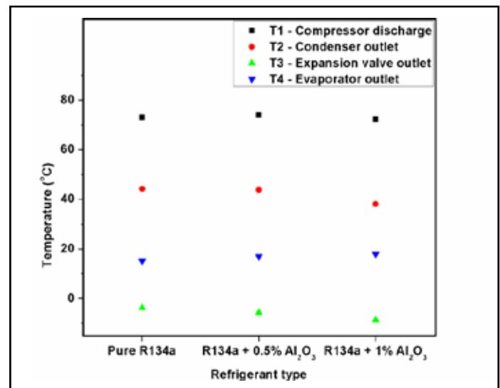
Fig. 5: Temperatures at Four Salient Points for Pure R134 and Nanorefrigerants at 16°C Evaporator Heat Load Temperature and 28°C Ambient Temperature
