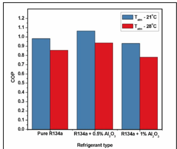
Fig. 2: COP Comparison for 6.5 LPH Volume Flow Rate, Evaporator Load at 15-17°C Operating at Ambient Temperature  $21^\circ\text{C}$  and  $28^\circ\text{C}$
