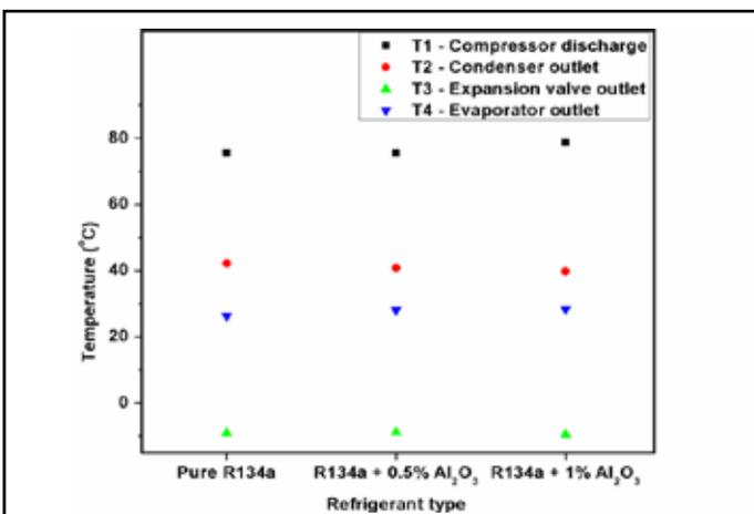
Fig. 7: Temperatures at Four Salient Points for Pure R134 and Nanorefrigerants at 30.5°C Evaporator Heat Load Temperature and 28°C Ambient Temperature
