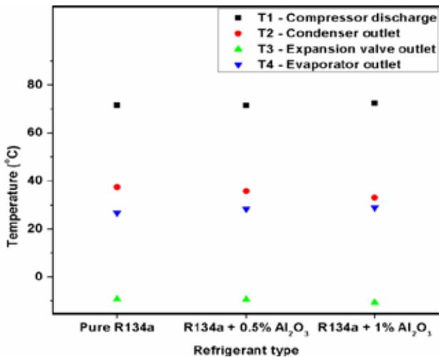
Fig. 6: Temperatures at Four Salient Points for Pure R134 and Nanorefrigerants at 30.5°C evaporator heat load temperature and 21°C Ambient Temperature
