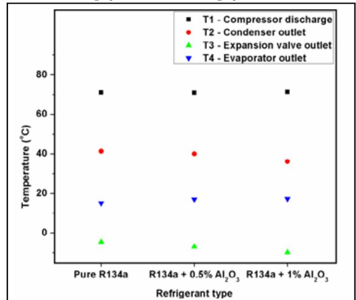
Fig. 4: Temperatures at Four Salient Points for Pure R134 and Nanorefrigerants at 16°C Evaporator Heat Load Temperature and 21°C Ambient Temperature
