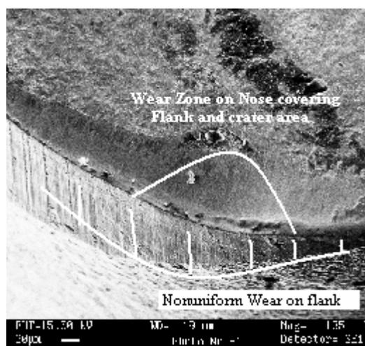
Fig. 1: Coated Carbide Tool After 6min of Machining at  $v=70$ m/min,  $f=0.08$ mm/rev and W.H=37HRC
