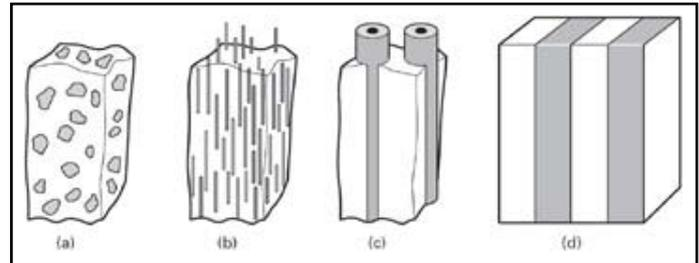
Fig. 1: Types of Metal Matrix Composites [2]
