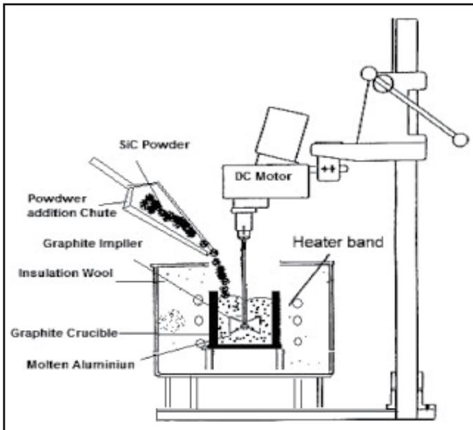
Fig. 2: Stir Casting by Vortex Method [3]
