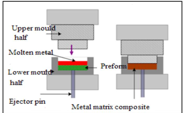
Fig. 4: Squeeze Casting [4]
