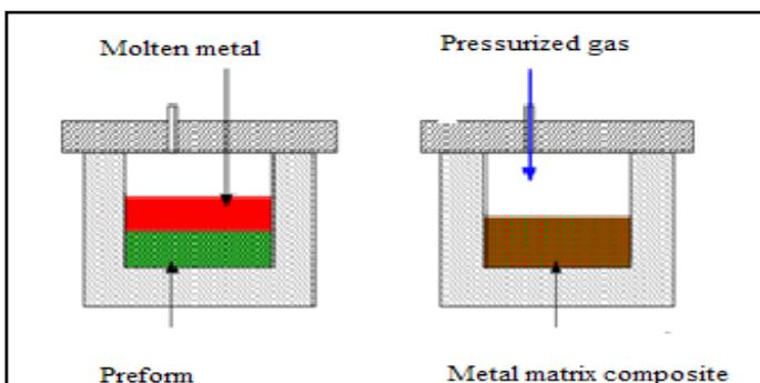
Fig. 3: Gas Pressure Infiltration [4]
