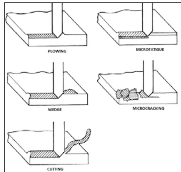
Fig. 1: Five Processes of Abrasive Wear [7]
