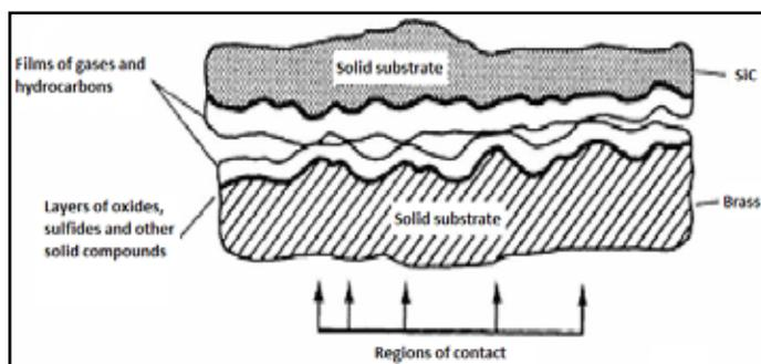
Fig. 2: Schematic of a bond bridge produced when two solid surfaces are in contact with each other [9].
