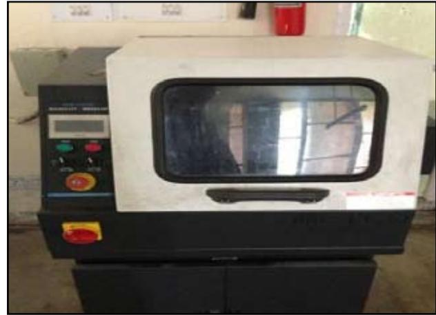
Fig. 3: Automatic Abrasive Cutting Machine Used for Cutting of Samples
