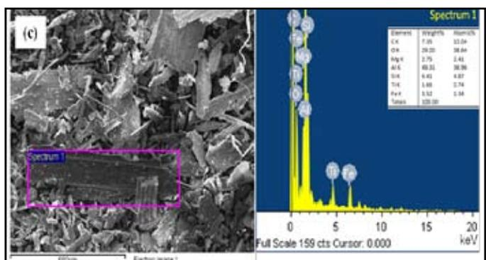
Fig. 3: SEM micrographs of composite-5C<sub>coarse</sub>: wear tracks (a) 9.8N, (b) 49N loads: EDS of wear track, and (c) debris at 49N loads.
