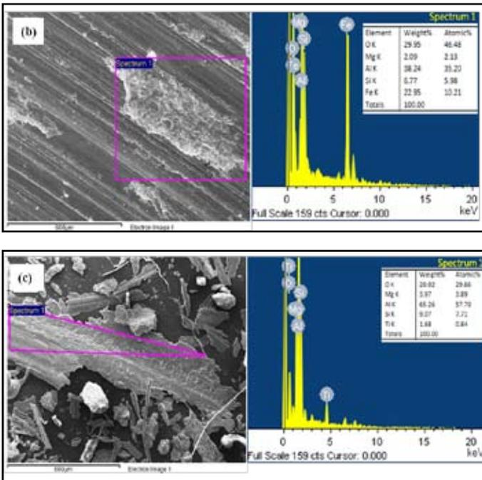
Fig. 4: SEM micrographs of composite- $^{10}\text{C}_{\text{coarse}}$ : wear tracks (a) 9.8N, (b) 49N loads: EDS of wear track, and (c) debris at 49N loads
