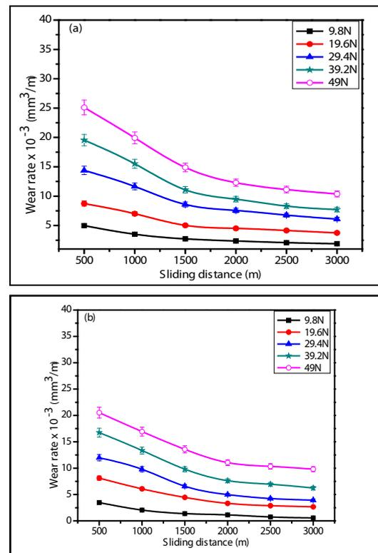
Fig. 2: Wear rate of rutile reinforced composites against sliding distance at different loads for (a) composite- ${}^5C_{\text{coarse}}$  and (b) composite- ${}^{10}C_{\text{coarse}}$
