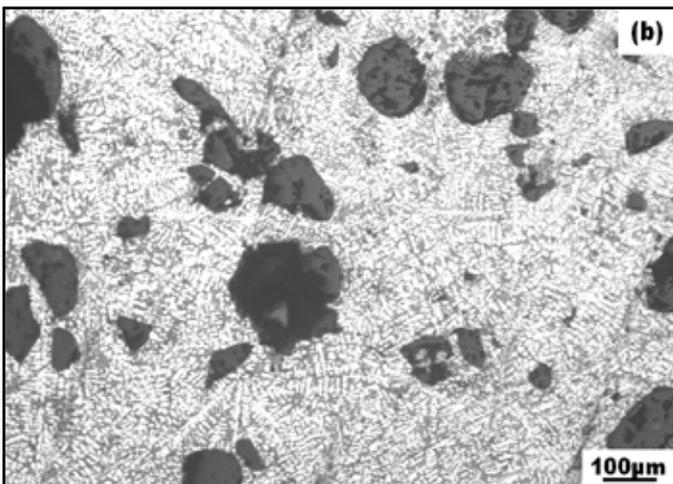
Fig. 1: The Optical Micrographs of Composite With Coarse Reinforced Size at Different Amount (a)  ${}^5C_{\text{coarse}}$  and (b)  ${}^{10}C_{\text{coarse}}$
