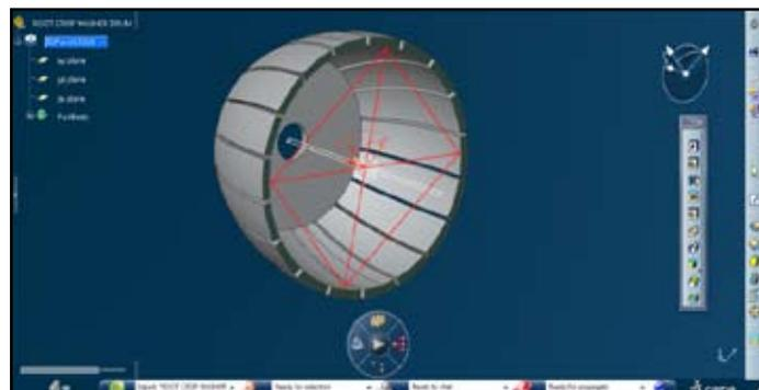
Fig. 2: Shows the Cross-Sectional View of the wooden Drum Used in the Automatic Root Crop Washer
