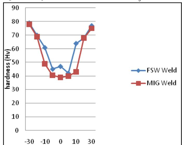
Fig. 3: Hardness Profile (Hv) FSW v/s MIG
