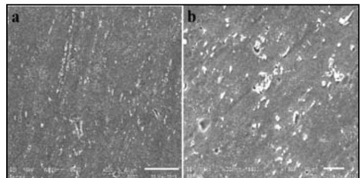
Fig. 8: SEM images of TMAZ of FSW at (a) 500X (b) 1500X
