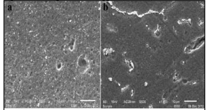
Fig. 7: SEM images of HAZ: a) FSW b) MIG
