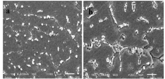
Fig. 6: SEM images of weld nugget: a) FSW, b) MIG
