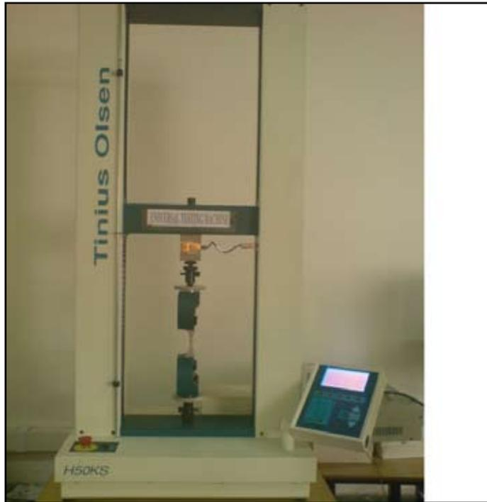
Fig. 2: Tensile Testing on UTM
