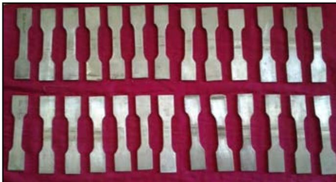
Fig. 5: Specimens Before Testing
