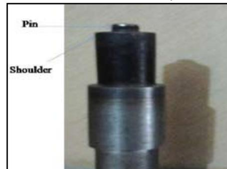
Fig. 2: Welding Tool Profile
