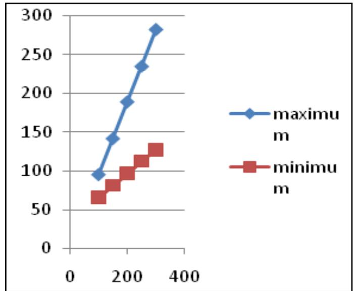
Graph 10: Graph of Concave Shaped Piston Crown Having Maximum Temperature, Minimum Temperature Versus Applied Load.
