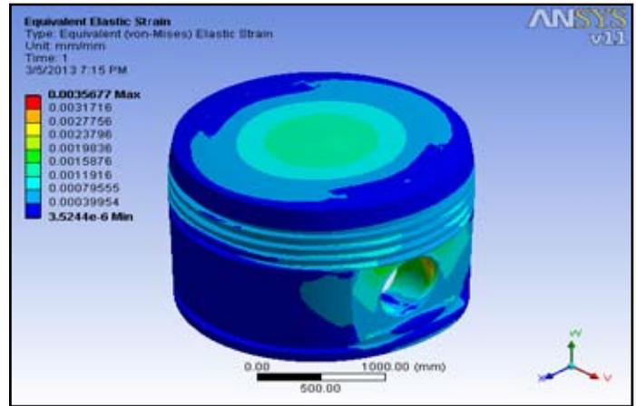
Fig. 8: Equivalent Strain Generated in the Concave Shaped Crown Piston
