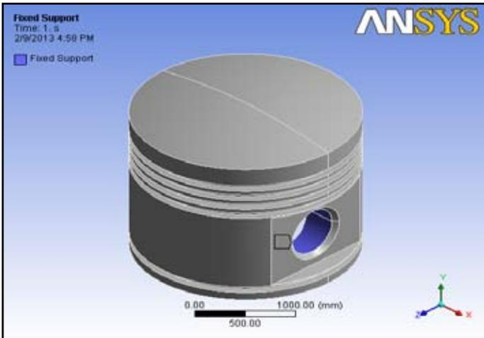
Fig. 5: Figure Shows the Boundary Conditions Applied For Piston
