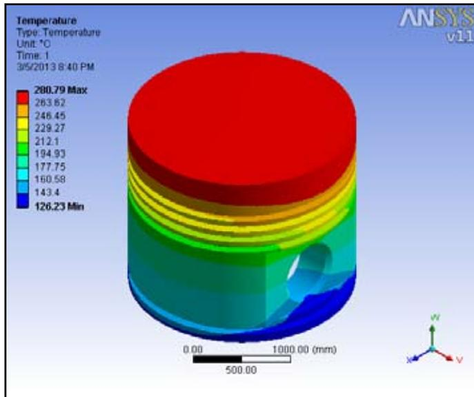
Fig. 20: Temperature Distribution for flat Shaped Crown Piston
