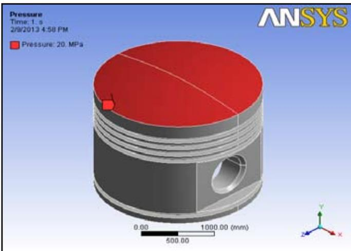
Fig. 6: Figure Shows Structural Load Acting on the Piston Head
