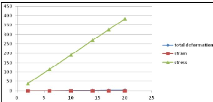
Graph 8: Graph Of Convex Shaped Piston Crown Having Total Deformations, Stresses, Strains Versus Loads
