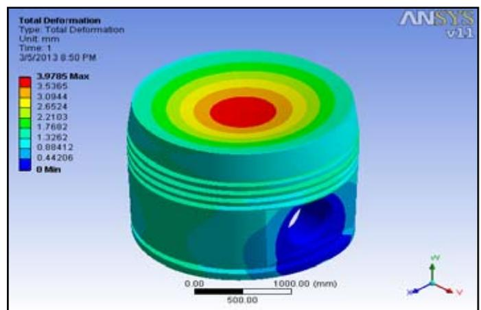
Fig. 10: Total Deformation for Convex Shaped Crown Piston
