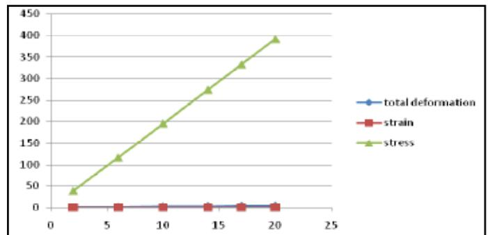
Graph 7: Graph of Concave Shaped Piston Crown Having Total Deformations, Stresses, Strains Versus Loads
