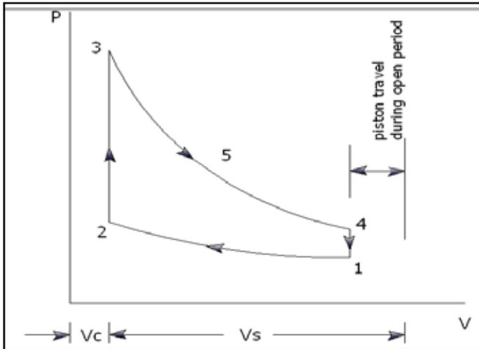
Fig. 1: Ideal Indicator Diagram of Two-Stroke SI Engine
