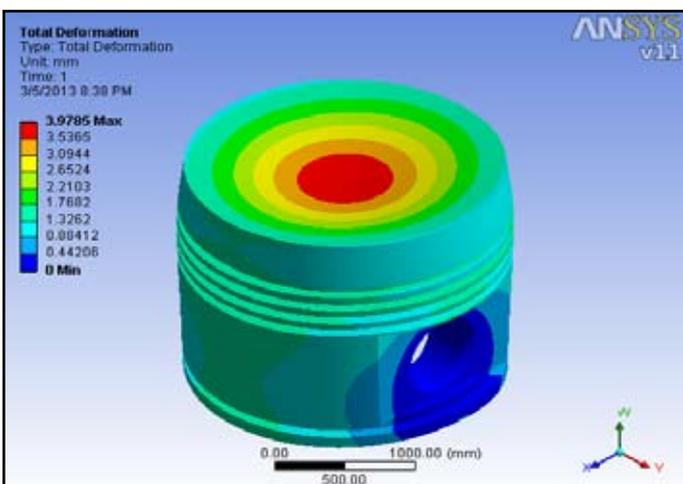
Fig. 13: Total Deformation for Flat Shaped Crown Piston
