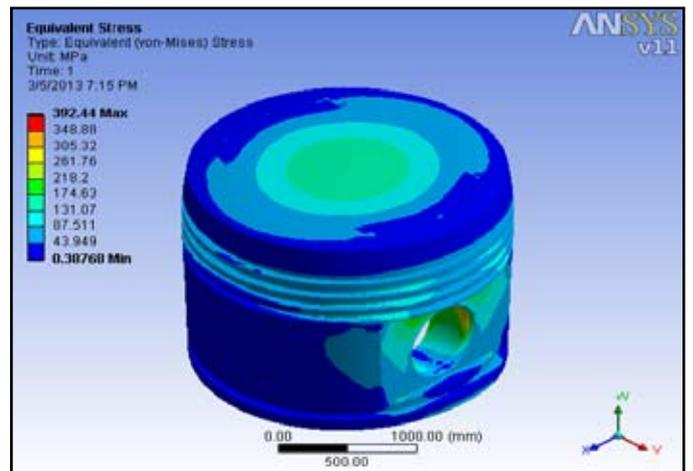
Fig. 9: Equivalent Stress Generated in the Concave Shaped Crown Piston
