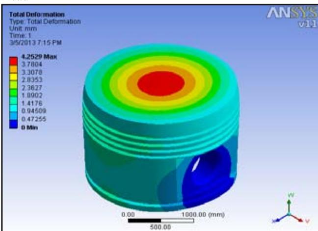
Fig. 7: Total Deformation for Concave Shaped Crown Piston
