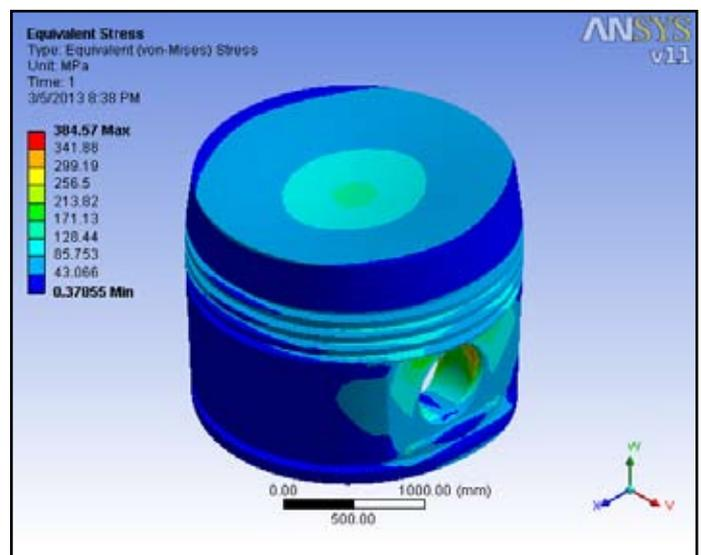
Fig. 15: Equivalent Stress Generated in the Flat Shaped Crown Piston
