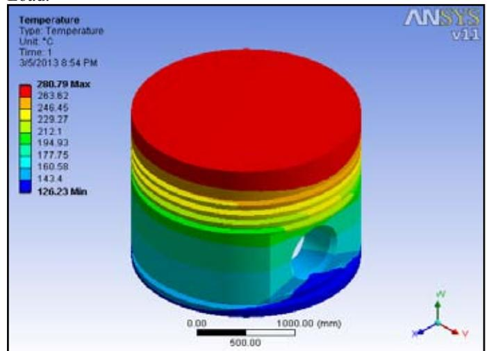
Fig. 18: Temperature Distribution for Convex Shaped Crown Piston
