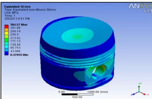
Fig. 12: Equivalent Stress Generated in the Convex Shaped Crown Piston
