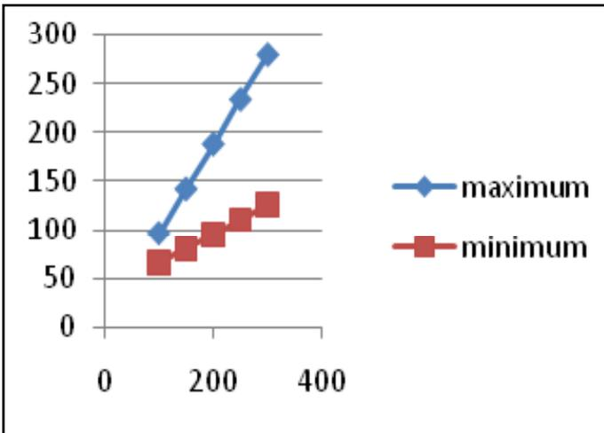
Graph 11: Graph of Convex Shaped Piston Crown Having Maximum Temperature, Minimum Temperature Versus Applied Load.
