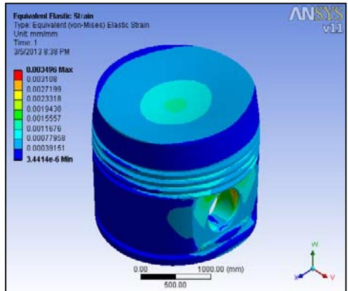
Fig. 14: Equivalent Strain Generated in the Flat Shaped Crown Piston
