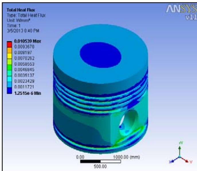
Fig. 21: Total Heat Flux for Flat Shaped Crown Piston
