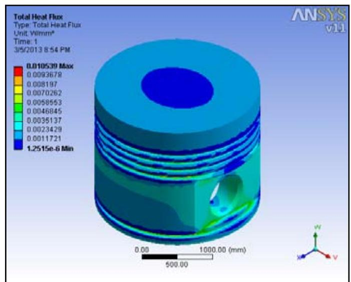
Fig. 19: Total Heat Flux for Convex Shaped Crown Piston
