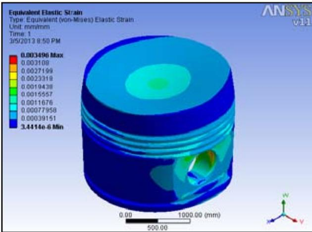
Fig. 11: Equivalent Strain Generated in the Convex Shaped Crown Piston
