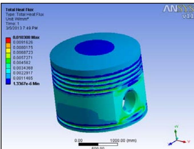
Fig. 17: Total Heat Flux for Concave Shaped Crown Piston
