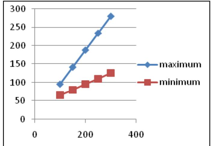
Graph 12: Graph of Flat Shaped Piston Crown Having Maximum Temperature, Minimum Temperature Versus Applied Load.
