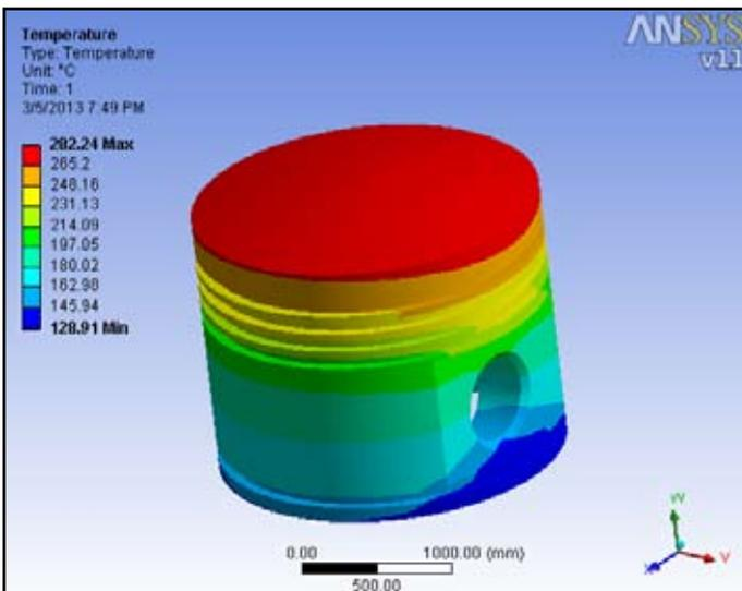
Fig. 16: Temperature Distribution for Concave Shaped Crown Piston
