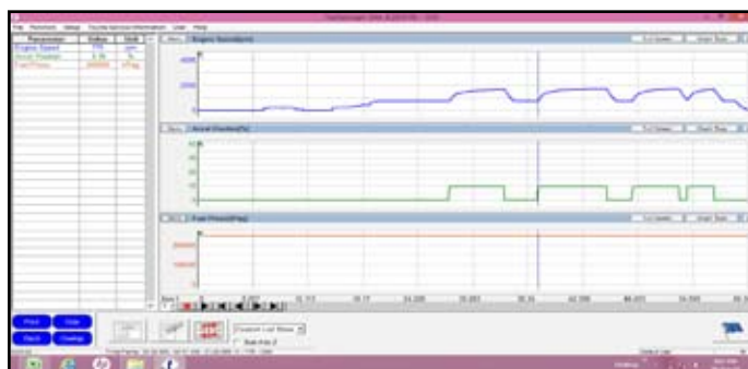
Fig. 2: Fuel Rail Pressure Sensor Circuit Faulty
