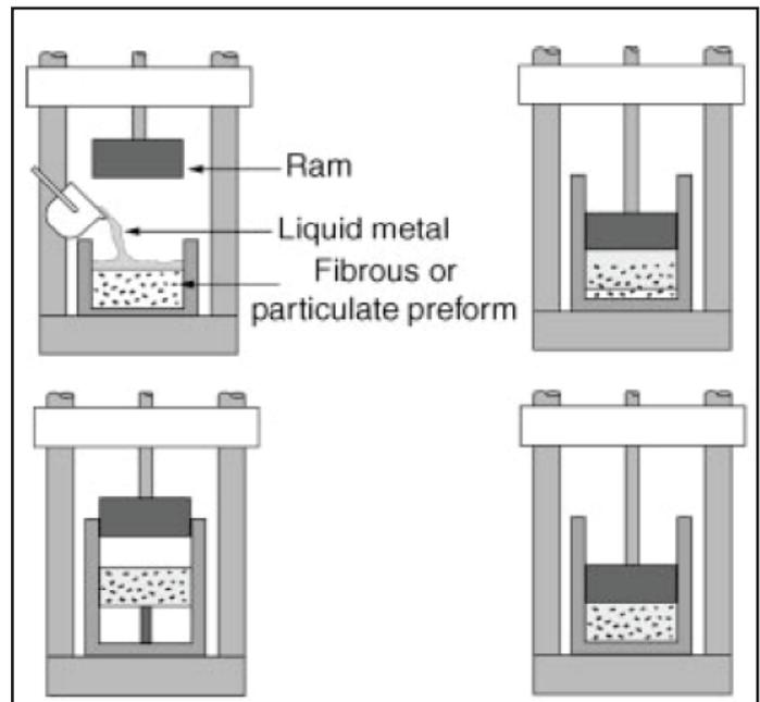
Fig. 2: Schematic Representation of Pressure Driven Infiltration
