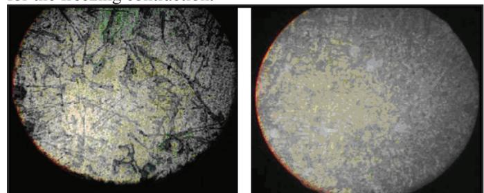
Fig. 3: Unreinforced Al-Si Alloy & Squeeze Cast Alloy
