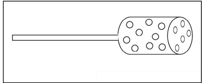
Fig. 1: Perforated Steel Capsule Welded to Plunger Rod
