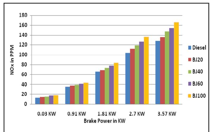
Fig. 9: Brake Power Vs NOx Emission
