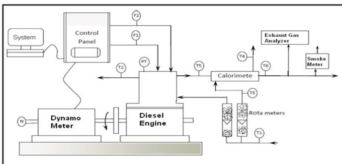
Fig. 2: Experimental Setup
