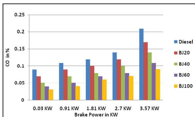
Fig. 3: Brake Power vs. CO Emission
