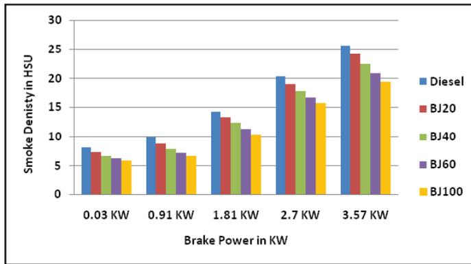
Fig. 5: Brake Power Vs Smoke Density
