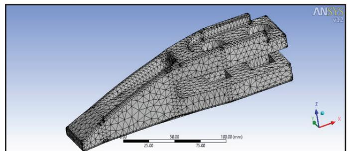
Fig. 2: Geometrical Model of Tooth of Meshing in Finite Element Analysis
