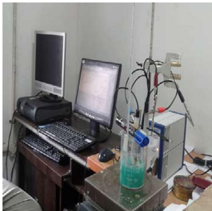
Fig. 1: Setup of Electro-Deposition Process
