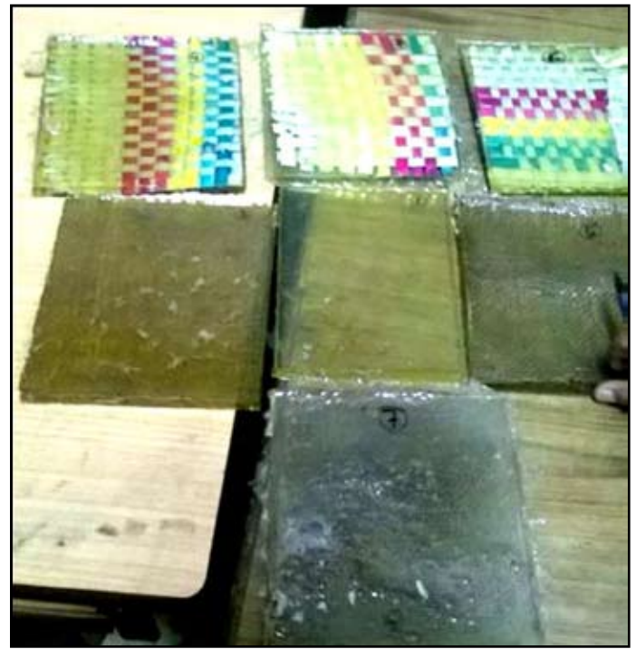
Fig. 2: Composite Hand Molded Laminate Sheets
