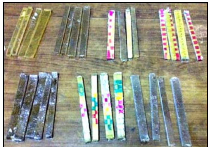
Fig. 3: Composite Specimens as per ASTM Standards for Tensile Strength
