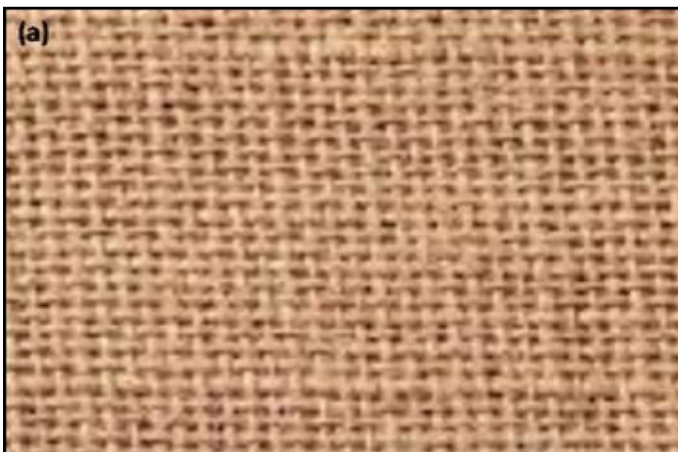
Fig. 1(a): Jute Bi-directional Woven Mat
