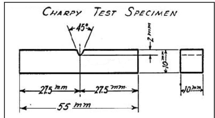
Fig. 3: Charpy Test Specimen Dimensions
