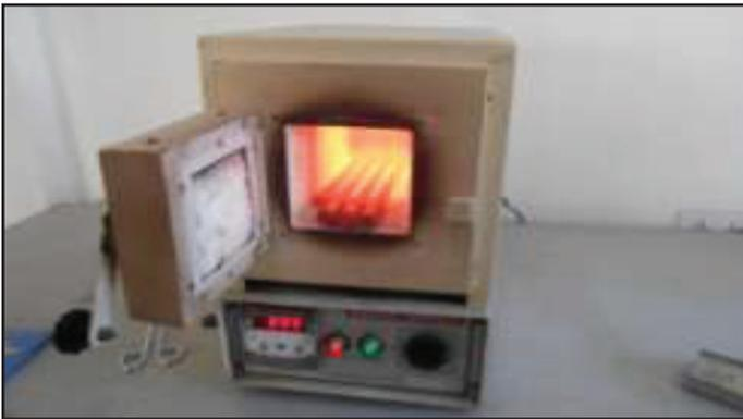
Fig. 2: Electric Muffle Furnace
