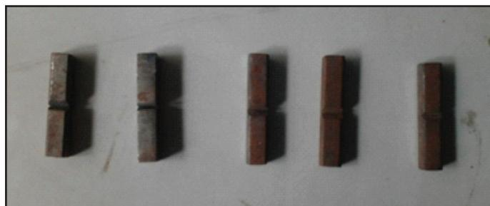
Fig. 1: Charpy Test Specimen Preparation
