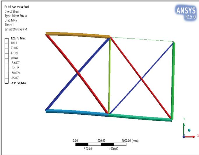
Fig. 8: Direct stresses in ten Bar Truss
