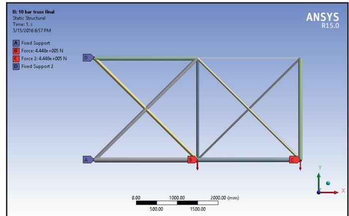
Fig. 17: Optimum Nine Bar Truss for Fabrication
