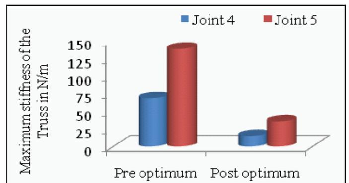
Fig 11. Reduced stiffness after optimization
