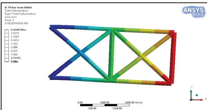
Fig. 4: Deformed Shape and Deflections
