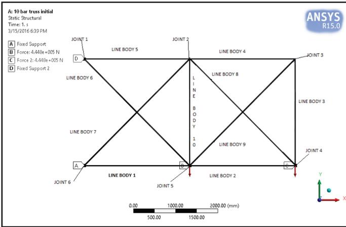
Fig. 2: Finite Element Model of of 10-bar Truss
