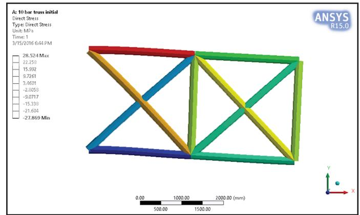
Fig. 5: Direct Stresses in Ten Bar Truss
