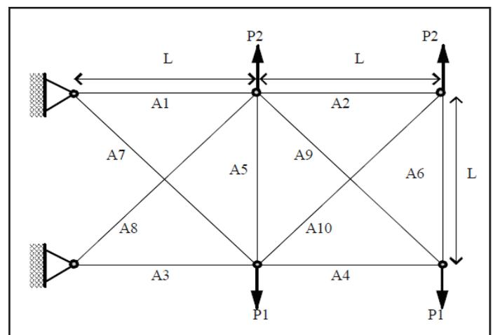
Fig. 1: Geometric Model of 10-bar Truss
