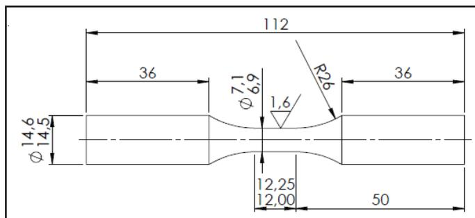
Fig. 2: Dimensions of Test Specimens, in Millimeters.
