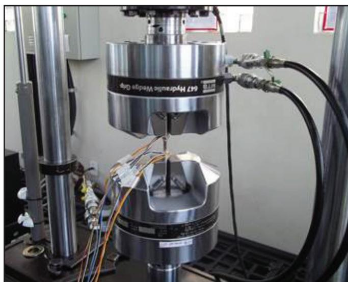
Fig. 4: Fixing System of the Specimens With Hydraulic Grips
