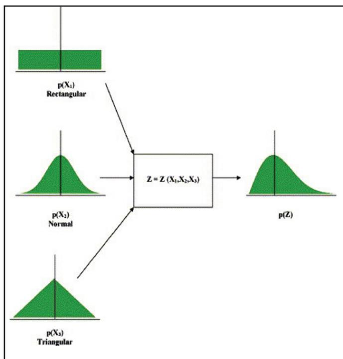
Fig. 1: Propagation of Distribution Through MCM [17].
