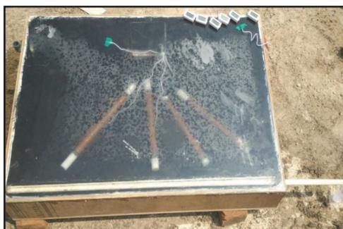
Fig. 2: Solar Still With PCM
