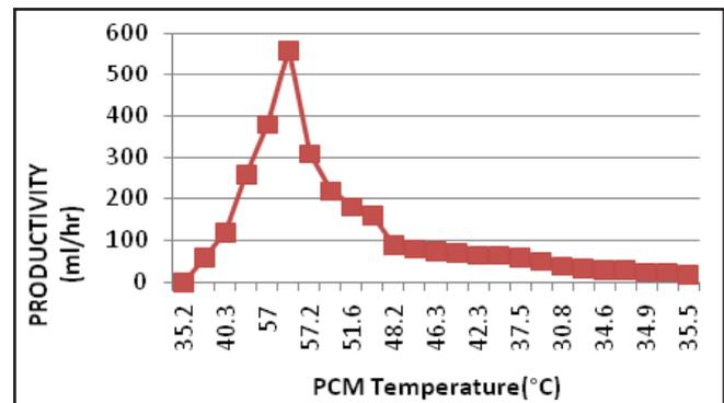
Fig. 6: Productivity With Respect to PCM Temperature (With PCM (Cetyl Alcohol))
