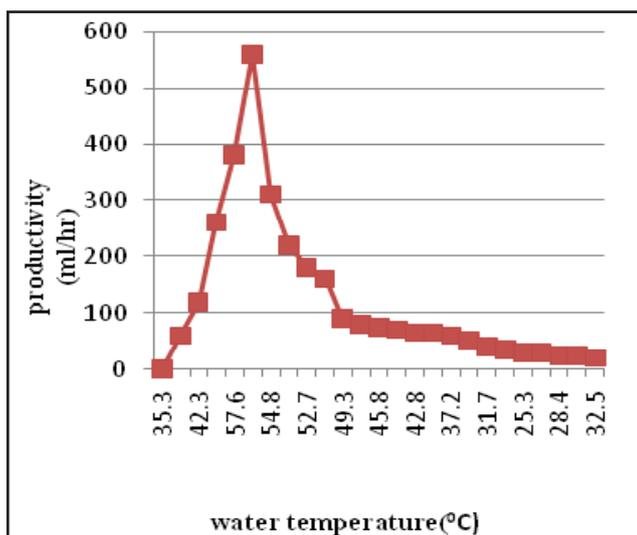
Fig. 4: Productivity With Respect to Water Temperature (With PCM (Cetyl Alcohol))
