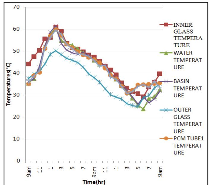
Fig. 5: Time With Respect to Different Temperature (With PCM (Cetyl Alcohol))
