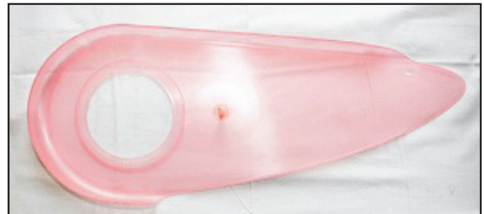
Fig. 12: The Component Produced From the Injection Mold.
