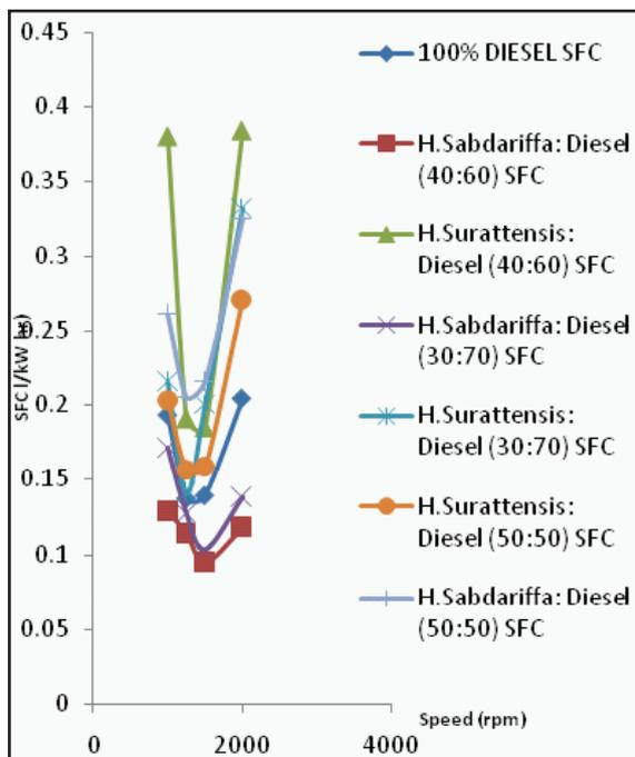
Fig. 5: Graph of Specific Fuel Consumption Vs Speed
