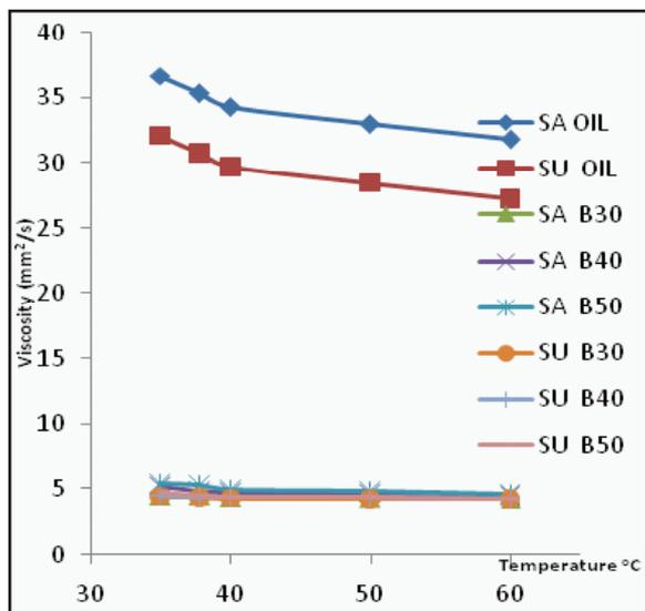
Fig. 1: Viscosity of the Various Biodiesel Blends
