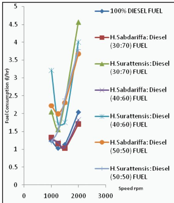
Fig. 4: Fuel Consumption for Different Speeds
