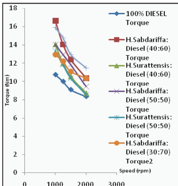
Fig. 2: Grph of Torque Vs Speed
