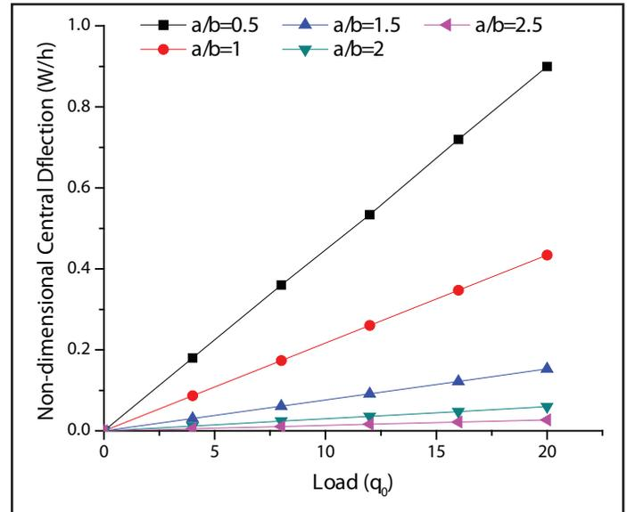
Fig. 6: Effect of Aspect Ratio on the Non-Dimensional Central Deflection in FG Sandwich Plate
