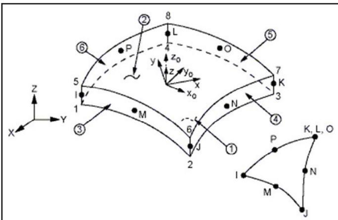
Fig. 2: Shell 281 Geometry (ANSYS 15.0)
