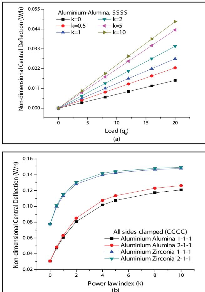
Fig. 4: Effect of power index (k) on the non-dimensional central deflection of FG sandwich plate.
