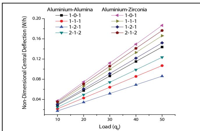
Fig. 5: Effect of Type of Symmetry on the Non-Dimensional Central Deflection of Aluminium-Alumina and Aluminium-Zirconia FG Sandwich Plate.
