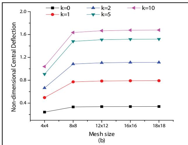
Fig. 3: Convergence Behaviour of Non-Dimensional Central Deflection of FG Sandwich Plate (a) Aluminium-Zirconia (for  $q_0=150\text{MPa}$ ) (b) Aluminium-Alumina (for  $q_0=1\text{MPa}$ ).
