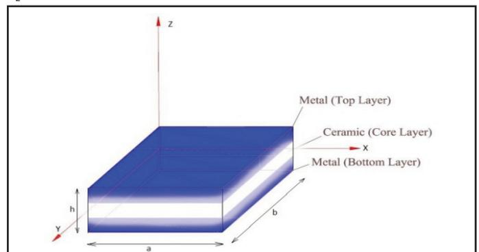
Fig. 1(a): Geometry and Dimensions of FG Sandwich Plate
