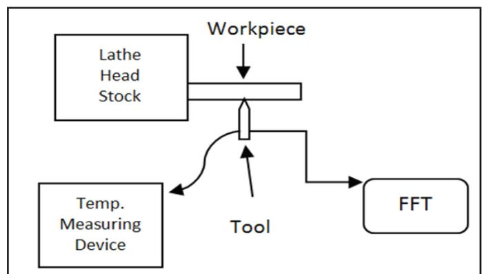
Fig. 3: Basic Block Diagram Of Experimental Setup
