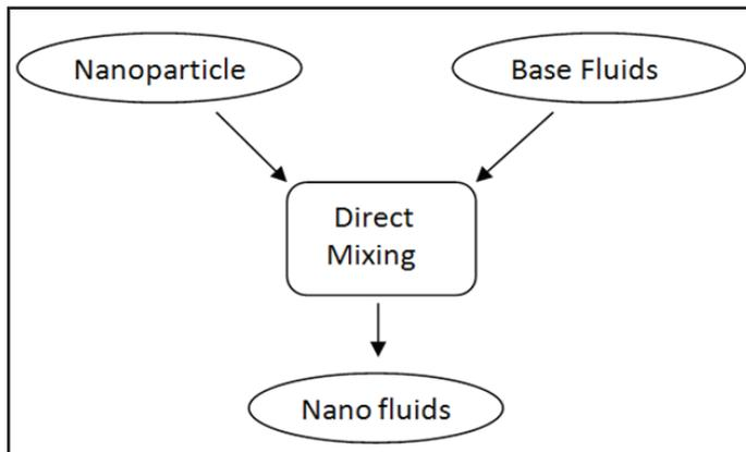
Fig. 1: Basic Block Diagram of Preparation of Nanofluid
