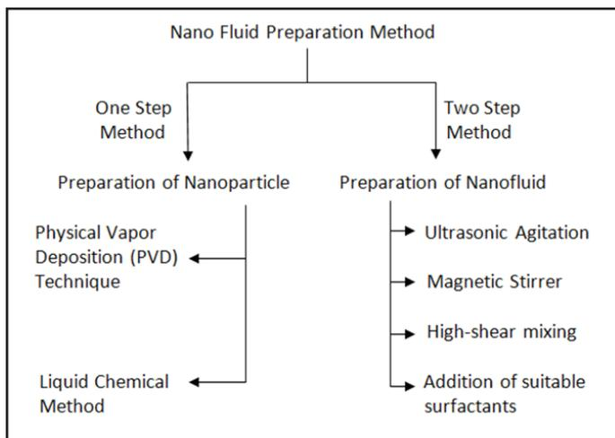
Fig. 2: Classification of Nano Fluid Preparation Method
