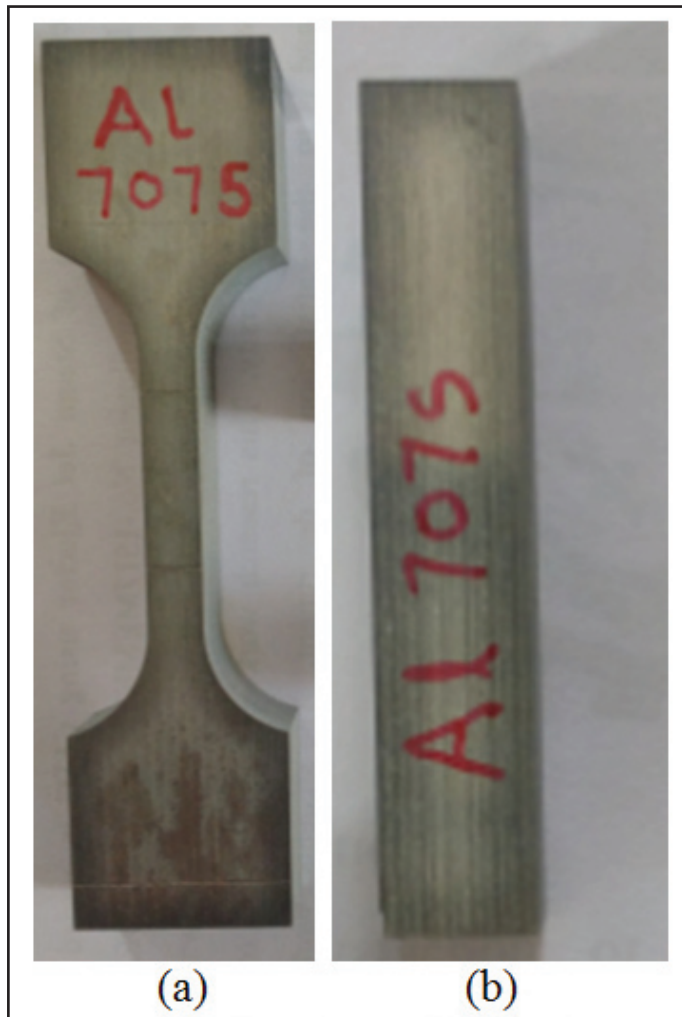
Fig. 3: Specimen for Mechanical Property Testing (a) Tensile Specimen (b) Hardness Specimen
