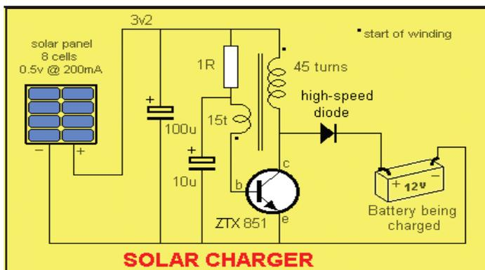
Fig. 2: Circuit Diagram for Solar Charger
