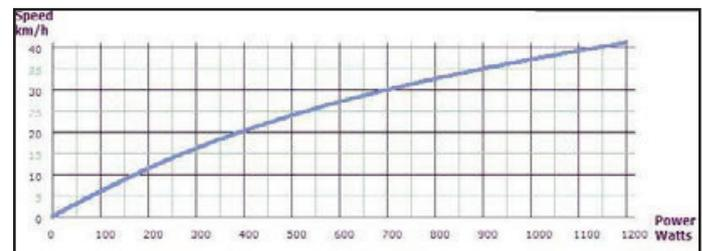
Fig. 5: Speed Vs Power on a flat Horizontal Road
