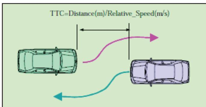
Fig. 10: TTC (Time To Collision) in which most drivers would not be able to avoid a crash even with a sudden avoiding operation
