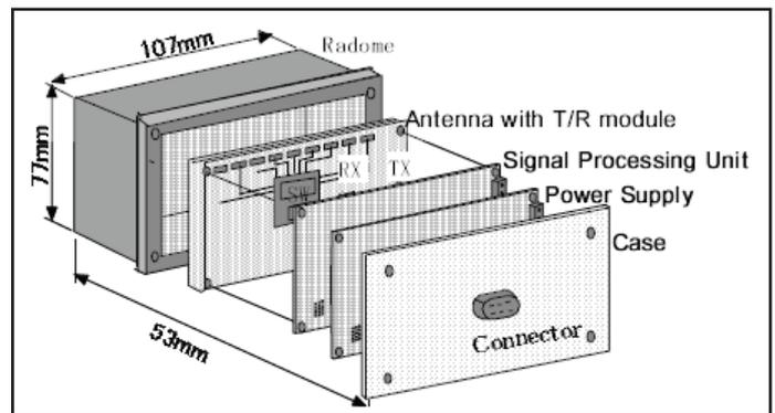
Fig. 6: Structure of Millimeter-Wave Radar
