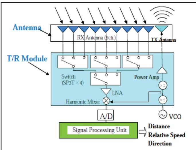
Fig. 4: Block Diagram of Millimeter-Wave Radar
