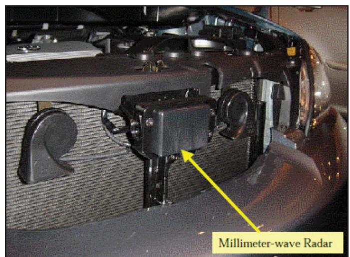
Fig. 7: Millimeter-Wave Radar Installed in a Vehicle
