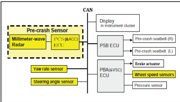
Fig. 3: Configuration of the Pre-Crash Sensor System
