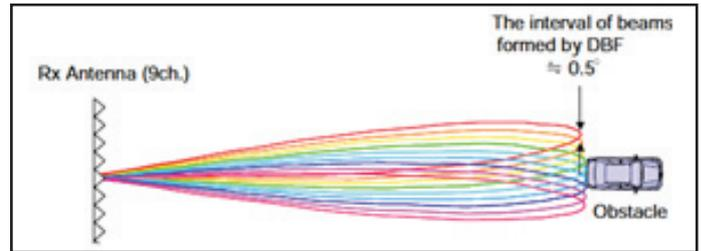
Fig. 5: Electronically Scanned Beams Using DBF (Digital Beam Forming) Technology
